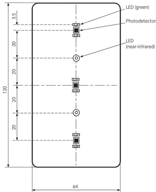
Fig 2: A schematic drawing of the photoplethysmography probe. Measurements are in mm. LED = light-emitting diode.
