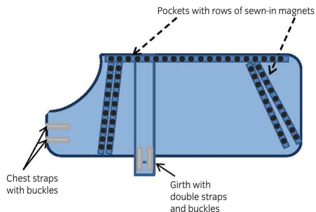
Fig 1: A schematic drawing of the magnetic blanket.
